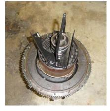
Bill ordered parts for reassembly. These included new brass screws to mount the magnets, and the spacers that the magnets rest on as well as shims for the coil ring. We found the magnet holders to be ok, and having heard bad things about the reproductions opted to re-use them.
